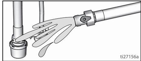
9. Unscrew inlet strainer from suction tube. Place inlet strainer in waste pail.
