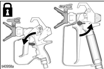
5. Remove tip guard. Do not lose the seal.
