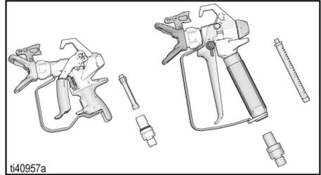
3. Remove spray tip and tip guard assembly and clean with water or flushing fluid and a brush.
