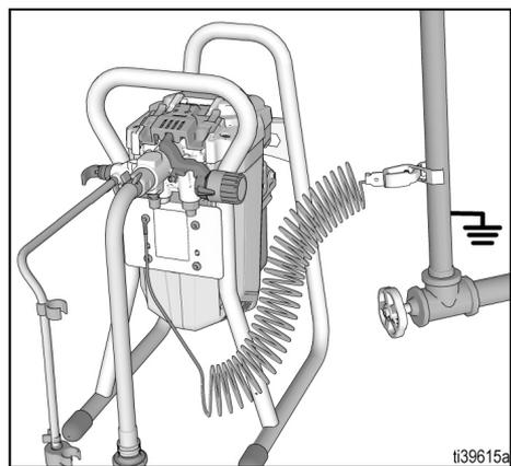
The sprayer is equipped with a grounding wire and clamp. The clamp must be connected to a true earth ground when spraying or flushing oil-based or flammable materials.
