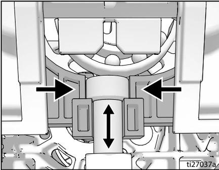
3. Swing easy access door pump door closed while pushing the entire door towards the inlet end of the pump.
