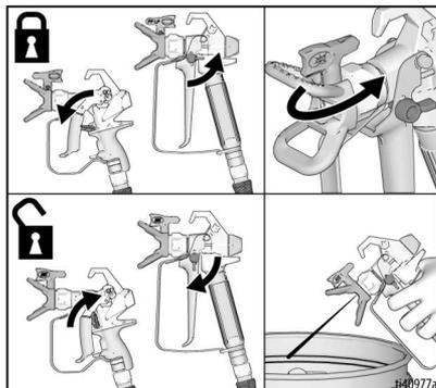
2. Engage trigger lock. Rotate spray tip back to spray position. Disengage trigger lock and continue spraying.
