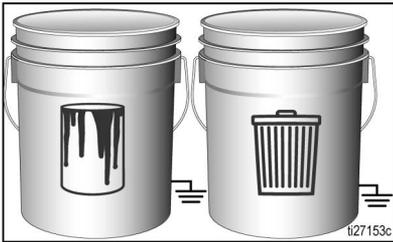
4. Lift suction tube and drain tube from paint pail. Let paint drain into the pail.
