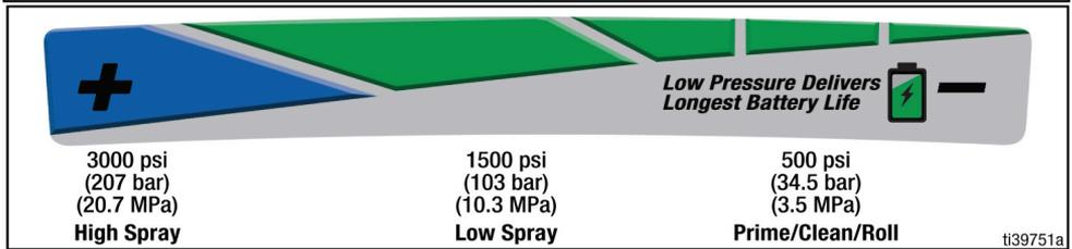
To select pressure, align symbol on pressure control knob with setting indicator on sprayer.
