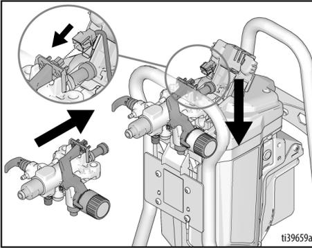
2. Move pump displacement rod up or down until cap is level with the opening in the yoke.
