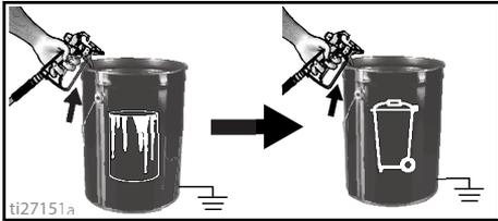
13. Stop triggering gun. Engage the trigger lock.
