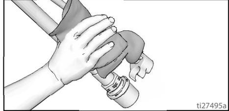
5. Separate drain tube (smaller) from suction tube (larger).
