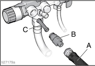
5. Check InstaClean Fluid Filter (C) for debris. If needed, clean filter with water or flushing solvent and a soft brush.
