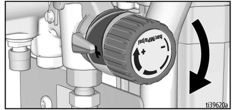
9. When sprayer starts pumping, flushing fluid and air bubbles will be purged from system. Allow fluid to flow out of drain tube into waste pail for 30 to 60 seconds.
