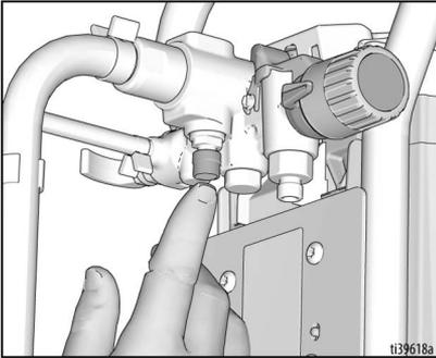
6. Align setting indicator with low setting on Pressure Control Knob.
