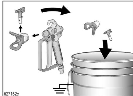
4. Wipe paint off outside of gun using a soft cloth moistened with water or flushing fluid.
