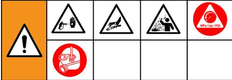
This equipment stays pressurized until pressure is manually relieved. To help prevent serious injury from pressurized fluid, such as skin injection or splashed fluid, follow the **Pressure Relief Procedure** whenever sprayer is stopped and before sprayer is cleaned or checked, and before equipment is serviced.
