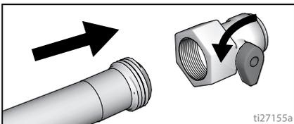
8. Turn on water. Open valve. Rinse paint off suction tube, drain tube and inlet strainer then close valve.
