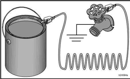
**To maintain ground continuity when sprayer is flushed or pressure is relieved:** hold metal part of spray gun firmly to the side of a grounded metal pail then trigger the gun.
