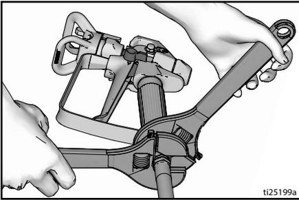
3. Use wrenches to tighten securely. If hose is already connected, make sure connections are tight.
