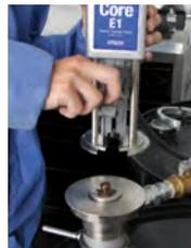
3. Slide Electric Motor to Remove
