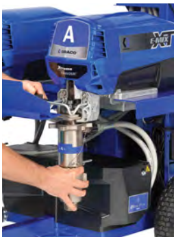
2. Open door and remove pump
