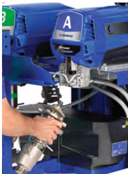
3. Remove hose and slide pump out
